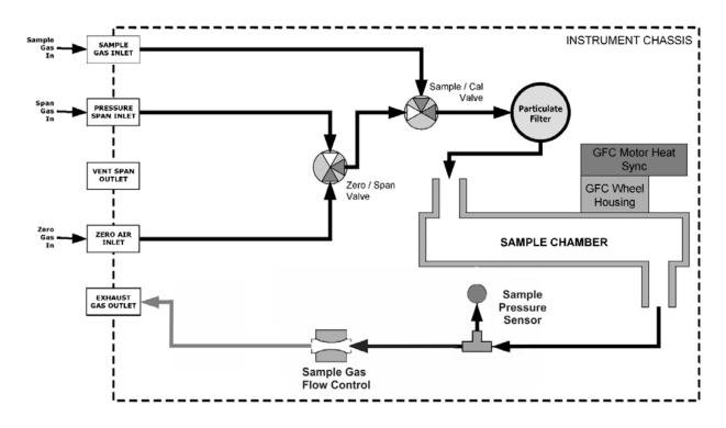
Figure 3-22 Internal Pneumatic Flow OPT 50A – Zero/Span Valves
